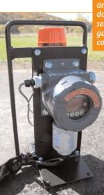
LEL Sensor provides real time digital readout of gas concentration and initiates alarm and/or auto shut down should gas level exceed selected thresholds. Operator adjusts gas/air mixing valve to maintain gas concentration well below LEL.
